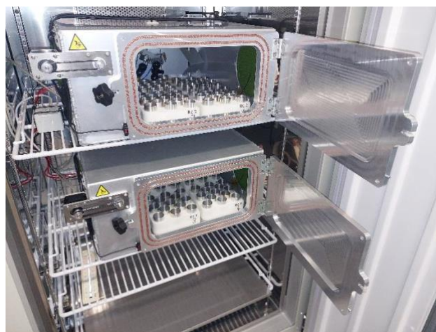
Figure 1: Reverberation chambers mounted inside the incubator, the vials with the drosophila are inserted into the metallic sample holder cups.
